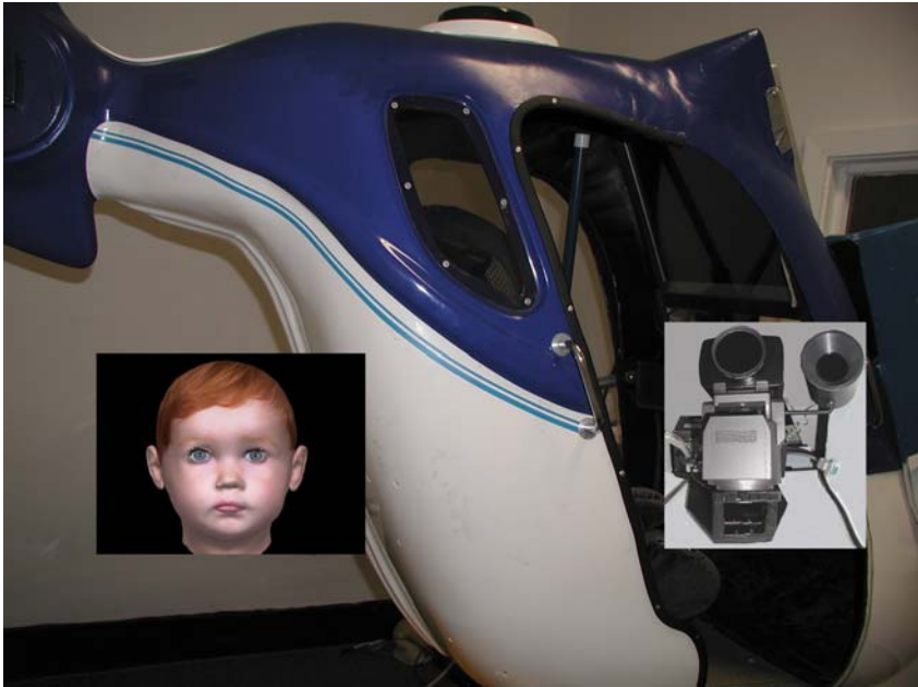
Fig. 11. A depiction of the ‘kiddie-ride’ training environment for the Autism Intervention Project. A camera inside the helicopter (inset on right) tracks eye-gaze as a child observes the screen. Interaction will take place with a ‘virtual buddy’ (inset on left) whose image is used to detect the child’s eye-gaze resulting in appropriate feedback
